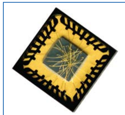
Figure 10. Example of a crossing insulated bonding wires in an open cavity QFN package.
