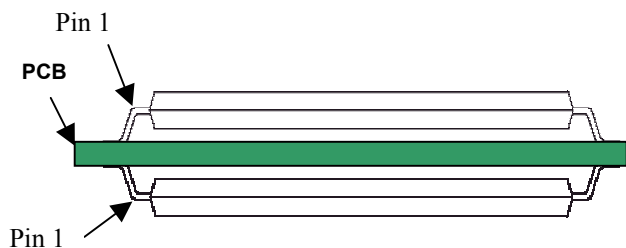
Figure 9. Bottom device gull wing leads are “reversed” formed in the opposite direction during trim and form.
